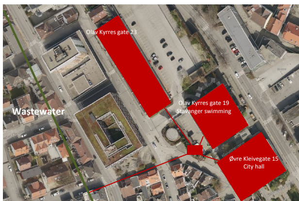
Figure 8 Energy from wastewater in municipal buildings in Stavanger city centre Source: Stavanger Municipality
